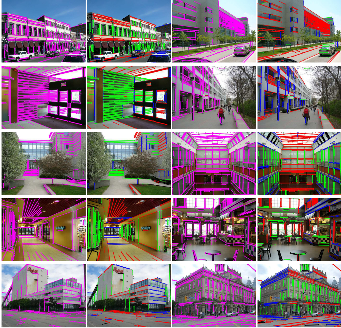
Figure 8. Vanishing point estimation results of the proposed method in the YUD dataset with line segments detected by the LSD [17]. The line segments detected by LSD are drawn in pink in the first and third columns, the line segments corresponding to different vanishing points are drawn in different colors and the outliers are marked in black in the second and fourth columns.
